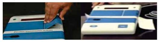
After Candidate set, seal cover of the Candidate Set Section of CU by passing a thread through hole provided on the right side using address tags showing the particulars of the election with the seal of the RO.
