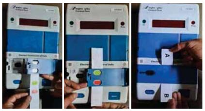
Fixing of Green Paper Seal and closing of inner compartment
