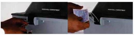
After installation of paper roll in the paper roll compartment of VVPAT, seal the latches of Paper Roll Compartment by passing a thread through holes provided on the latches using Address Tag showing the particulars of the election with the seal of the RO.
