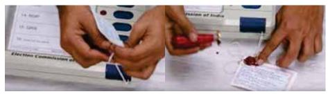
After unmasking candidate buttons, seal the upper cover of the BU by thread passed through holes on the top and bottom end at right side using address tags showing the particulars of the election with the seal of the RO.
